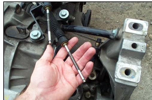
Figure 23 - Expose All of the Threads and Smooth Cable
