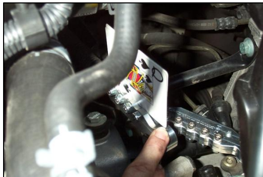
Figure 49 - Two Playing Cards Will Fit in the Gap
