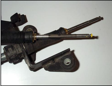
Figure 20 - Expose All Threads of this Cable
