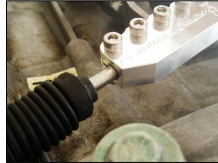
Figure 27 - Make Sure the Cable Can Be Inserted into the Cable End Until the Threads Disappear
