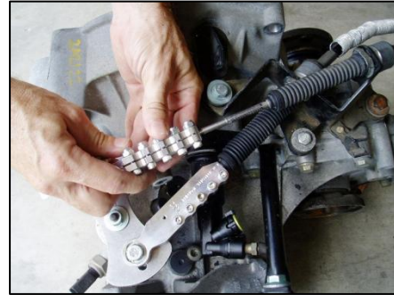
Figure 38 - Take the Remaining Silver Side to Side Shift Bracket and Engage the Lubricated Shift Cable with the Aluminum Cable End
