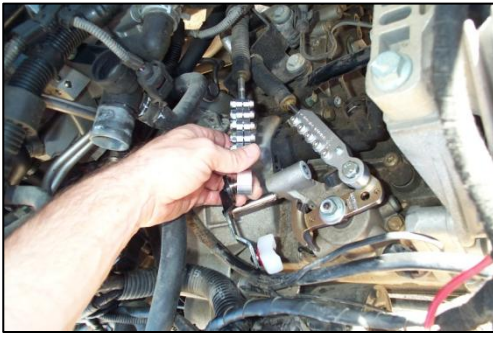
Figure 39 - Position The Side To Side Bracket Cable End Back Just Far Enough To Expose All Of The Shift Cable Threads
