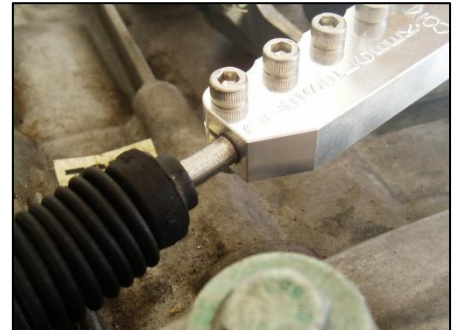
Figure 34 - The End of the Threads of the Shift Cable Are Roughly Even with the Opening of the Aluminum Cable End
