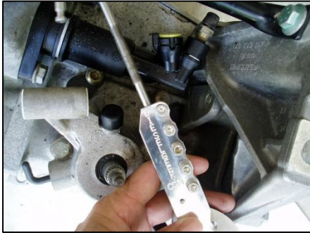
Figure 26 – Slide the Aluminum Cable End Onto the Lubricated and Partially Threaded Shift Cable
