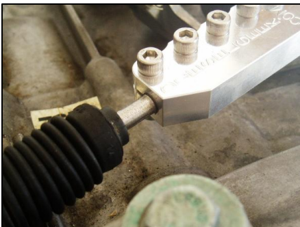
Figure 18 - Slide the Cable End Freely Onto the Shift Cable Until the Threads Disappear
