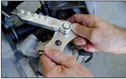
Figure 30 - The Shift Bracket Will Push Onto the Selector Shaft
