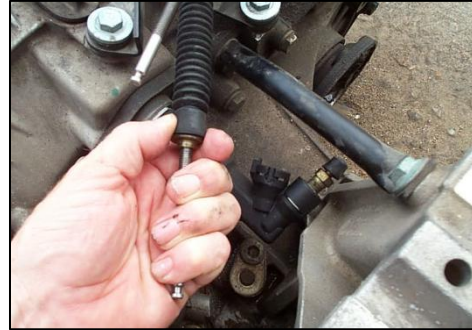
Figure 21 - Pull the Plastic Ring Toward the Front of the Car
