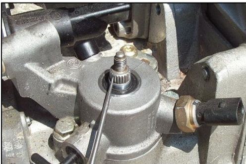
Figure 28 - Keyway or Joined Spline On the Selector Shaft On the Transmission
