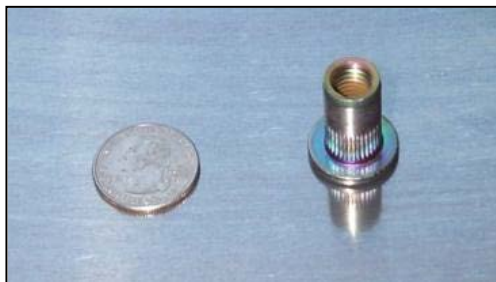
Figure 7a - Silver Colored Rivnut, Figure 7b - Black Colored Rivnut
