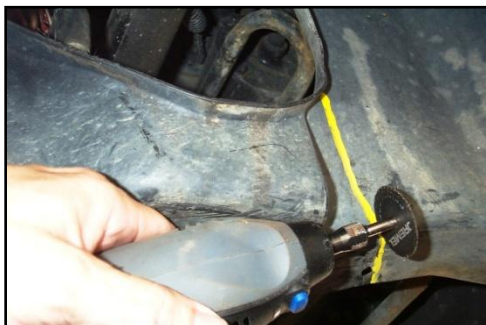
Figure 13 – Using Dremel Tool to Cut Side Panel
