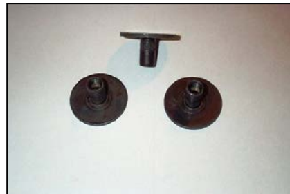
Figure 7a - Silver Colored Rivnut, Figure 7b - Black Colored Rivnut
