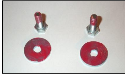
Figure 32 – Greased 10mm Bolts
