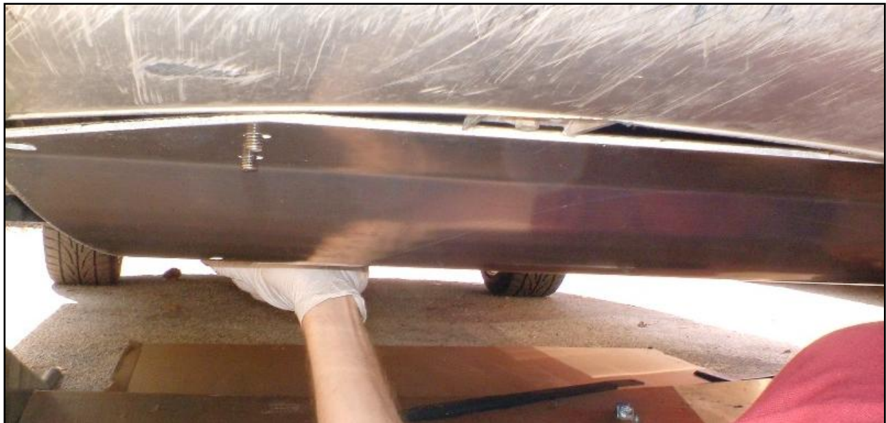
Figure 36 – Lining up the Skid Plate
