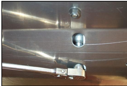
Figure 37 – Two Oblong Holes in the Skid Plate
