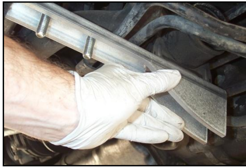
Figure 26 - Engage the U-Bolt Studs with the Aluminum Mounting Bracket
