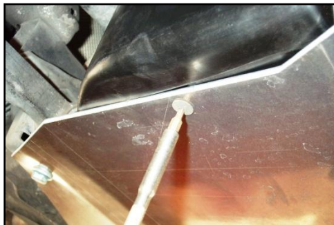
Figure 38 - Attaching the Vertical Engine Bay Side Panels
