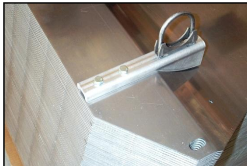
Figure 21 - Custom Aluminum Bracket
