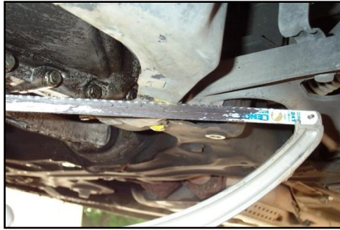
Figure 11- Using a Hack Saw to Cut the Side Panel
