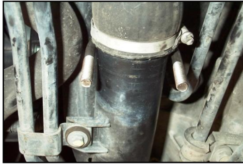
Figure 22 - Exhaust Clamp U-Bolt over the Steel Intercooler Tube
