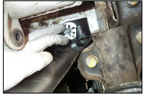
Figure 20 - Star Washers of the New Side Panel on the Threaded Stud Mounts
