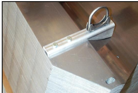
Figure 20 - Custom Aluminum Bracket
