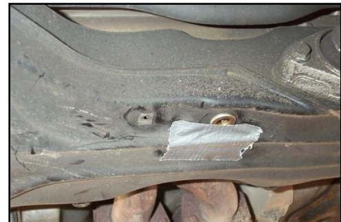
Figure 33 - Use a Small Piece of Duct Tape to Fix Rivnut in Place
