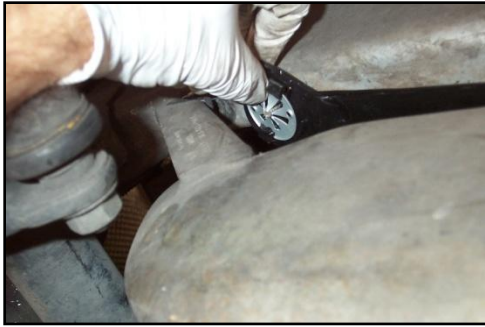
Figure 18 – Installing Star Washers
