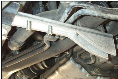
Figure 26 - Thin End Forward and Even With the Radiator Support.
