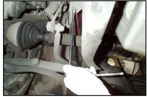
Figure 15 – Removing the Sheetmetal Nut
