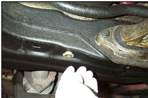
Figure 32 - Rivnut Staying In the Hole
