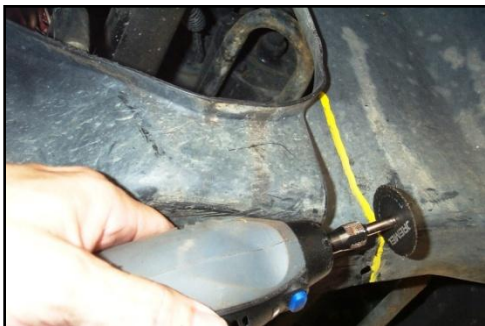
Figure 12 – Using Dremel Tool to Cut Side Panel
