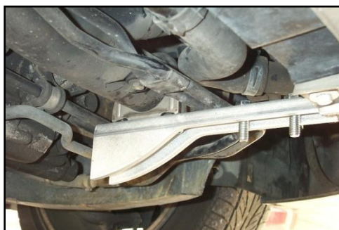
Figure 23 - Custom Aluminum Bracket
