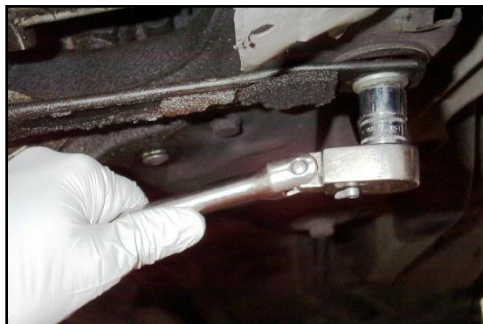
Figure 28 - Removing the Flattened Black Steel Original Equipment Stress Bar
