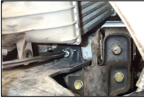
Figure 14 – Location of the Sheetmetal Nut
