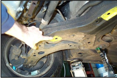
Figure 30 – Pre-existing 13mm holes on the car's subframe (passenger side)
