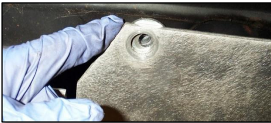
Figure 56 - Slip the last extra washer between the skid plate and the rear center bolt hole
