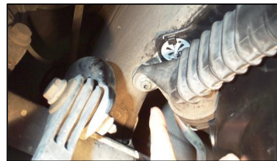
Figure 29 - 6mm nut holding the rear of the intercooler pipe (10mm wrench required)
