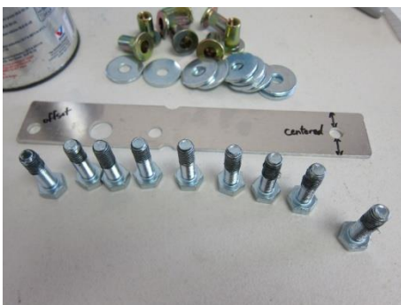
Figure 36 - Greasing the bolts
