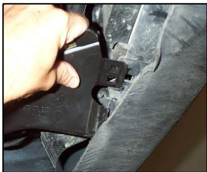
Figure 53 - Sliding the front rounded edge into the slot in the radiator support
