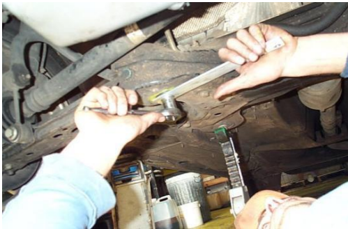
Figure 39 - Tighten the 10mm bolt
