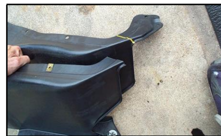
Figure 52 - The final cut is simply removing the tail section
