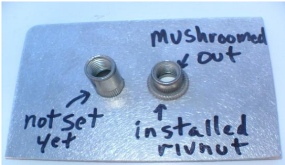
Figure 40 - The rivnut will mushroom out and expand
