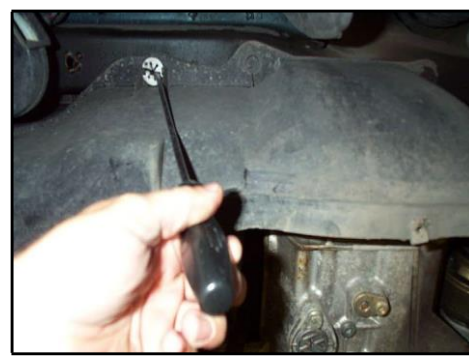
Figure 55 - Tighten the star nuts further by placing a flat bladed screwdriver in one of the star nut's
