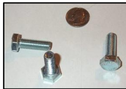
Figure 2 - 35mm long bolts
