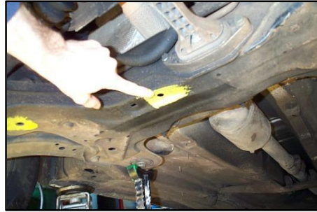
Figure 31 – Pre-existing 13mm holes on the car's subframe (center)
