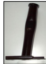
Figure 49 - The post is not welded perpendicular to the base plate
