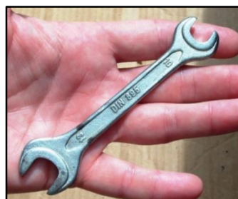
Figure 25 - Combo wrench (from the VW tire change tool kit in the trunk)
