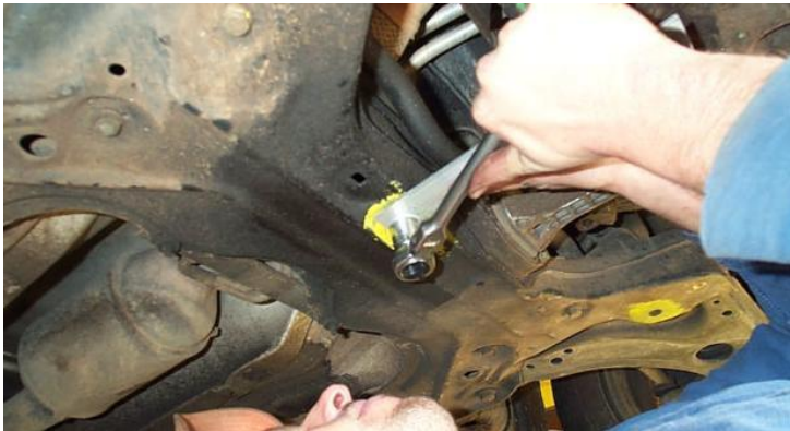
Figure 40 - The rivnut will mushroom out and expand
