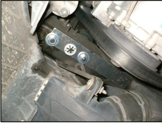
Figure 45 - The "tail" of the rivnut tool will go toward the rear of the car
