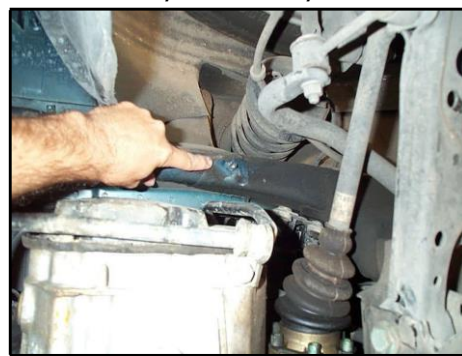
Figure 54 - Pushing their star nuts onto the threaded stud on the bottom side of the frame rail
