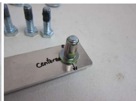
Figure 38 – Thread Rivnut on
